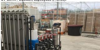
Closed loop water filtration for tomato irrigation in a greenhouse. Filtration 20 µm before UV system.
